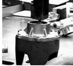
6. With the rollers exposed, remove them. When replacing damaged rollers, always replace the full set.
