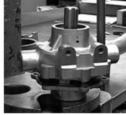
**ATTENTION:** Before new parts are installed, all burrs should be removed, particularly in the rotor slots and body. Do not machine clean the body casting. A more satisfactory job can be done by hand cleaning with an emery cloth.
