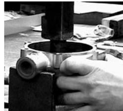
10. To press the shaft out of the rotor, first carefully wash the rotor and shaft - removing all traces of rust and other foreign matter. Use steel wool or emery cloth, rinsing parts afterward to wash off all emery dust. Remove the Allen set screw. Support the rotor in the press through the slot in the base and press shaft through.
