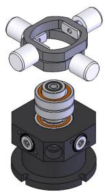
5. Remove bolts and then retaining plate from head. Remove guide, seal ring, and O-ring from head.
