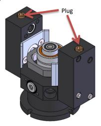
12. Flip other hoop assembly so plugs are down. Slide hoop onto driveshaft. Start bottom bolts on heads.
