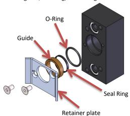
6. Grease seal ring and O-ring. Place O-ring into head. Slide retainer plate, guide, and then seal ring onto the plunger and install into head.
