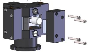
3. The inlet manifold can now be removed by lifting them off of the driveshaft.
