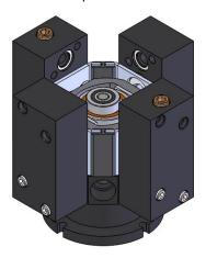
14. Pull heads apart slightly. Note orientation of inlet is opposite of outlet before sliding manifold into place. Slide inlet manifold with bearing housing onto top of driveshaft.
