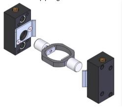
11. Slide hoop plunger/head assembly onto driveshaft with the plugs facing up. Start bottom bolts on heads.
