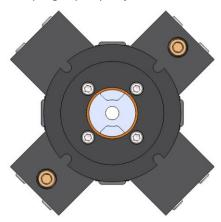
18. Slide pump onto motor and tighten flange head bolts.
