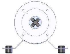
17. Orient coupling in pump so jaws are vertical.
