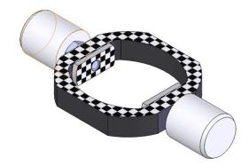
10. Place one head onto each end of plunger hoop. Do this for both hoop plungers.
