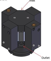
15. Push heads together onto manifolds. Manifold should slide easily and completely over valves. Insert and tighten bolts in each head in order shown below. Tighten 1<sup>st</sup> bolt again after 4<sup>th</sup> bolt is tightened.
