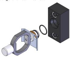
7. Tighten bolts to secure retainer plate. Remove hoop plunger. Replace valve washers if needed. A small amount of grease helps keep the washers in the pockets. Repeat steps 5, 6, and 7 for other three heads.
