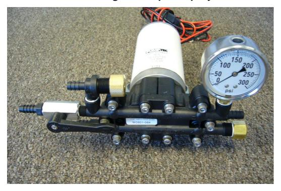
Spray Basic has 1 Inlet (suction) ports and 2 outlet (pressure) ports.
