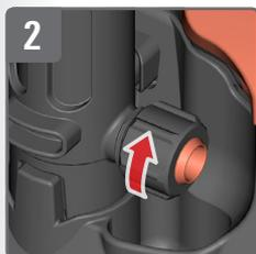
**2** Screw in grease cup clockwise 1/4 turn
