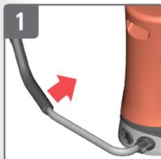
**1** Bring pump lever into raised working position
