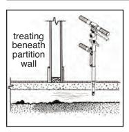
$360^{\circ}$  spray = 2 gal/min  $180^{\circ}$  spray = 2 gal/min
