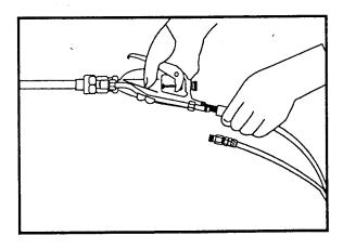
stainless steel air line (part number 26), allowing the air line side of the plastic hose to hang free. Now the strainer housing (part number 15) can be removed without twisting or knotting the hose.
